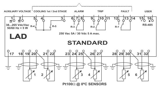
The function of each relay is user configurable. The values below are the factory default.
